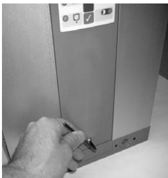
6. Replace single retaining screw.
