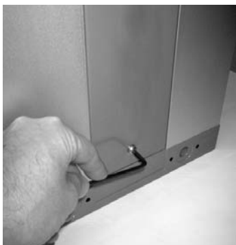
2. Remove single retaining screw.
