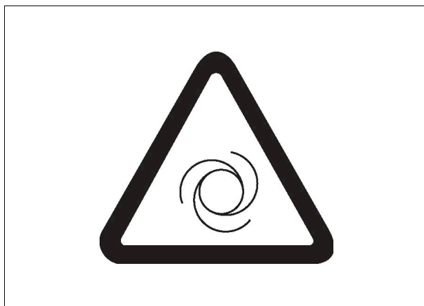
This system can start up by means of a remote control or automatically after a power failure.
