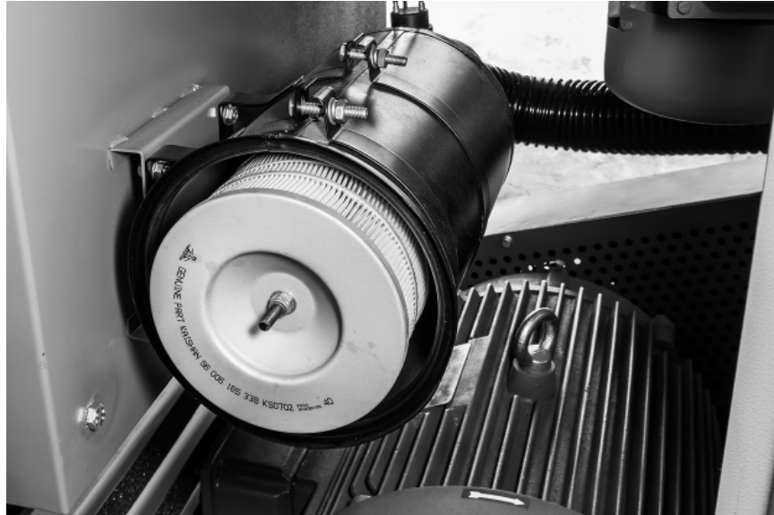
Figure 2. KI and KIV Air Inlet Filter Removal.
