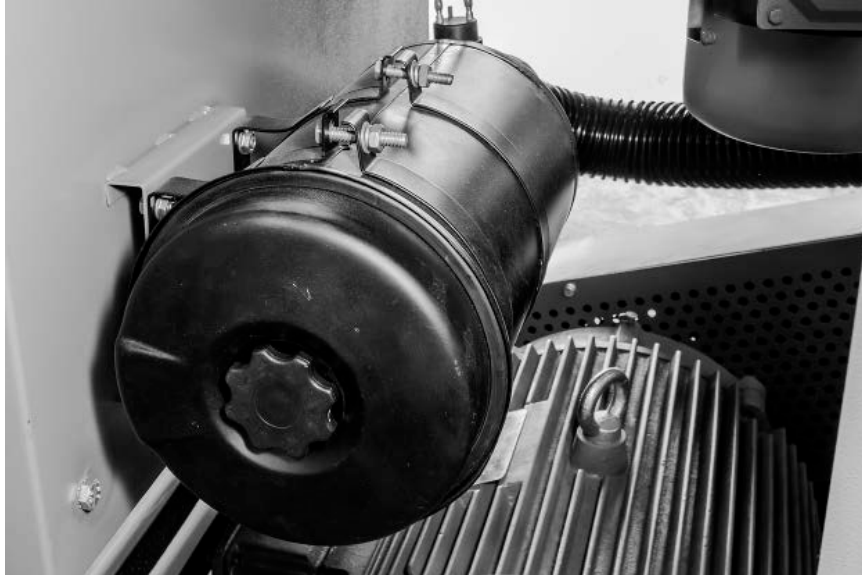
Figure 1. KI and KIV Air Inlet Filter Housing (typical).
