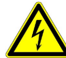
High Voltage – Hazard of Shock, Burn, or Death Present until Electrical Power is Removed
