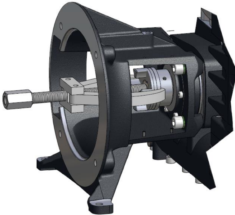
Figure 8-4 – COUPLING REMOVAL TOOL
